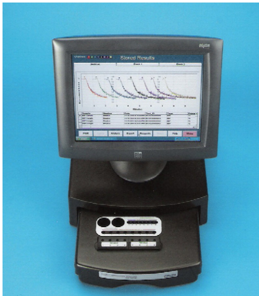
Figure 1 An example of a modern 8-channel platelet aggregometer. The model shown is the Biodata PAP-8E. Reproduced with permission from Biodata and Biodis.
