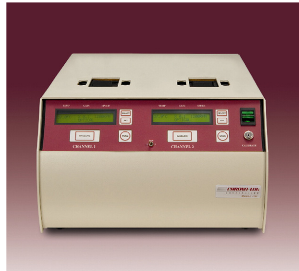
Figure 2 The Chrono-log Model 700 whole blood/optical 2 channel lumiaggregometer. Reproduced with permission from Chrono-log.
